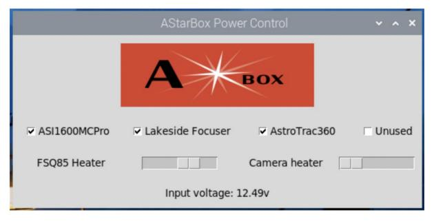
The names and power states are persistent. When you turn on your AStarBox, the power states will be restored to their last settings. In this case, the ASI1600MCPro, Lakeside Focuser and AstroTrac360 will be turned on, the FSQ85 dew heater will be set to about 65% power and the camera heater will be switched off.
