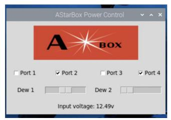
Clicking on the radio buttons will turn the power on and off. The amount of power going to the dew heaters is controlled by the sliders. Here Ports 2 and 4 are on, while Dew 1 is at about 50% power and Dew 2 is off. The control panel also shows the input voltage. The port and dew controller numbers correspond to those on the AStarBox case:
