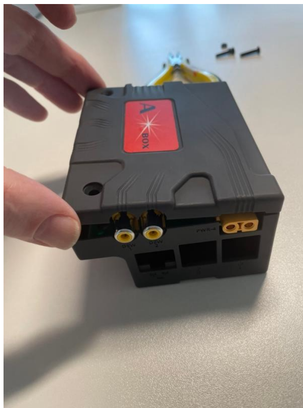
Figure 5. Remove the top of the case by lifting as shown.
