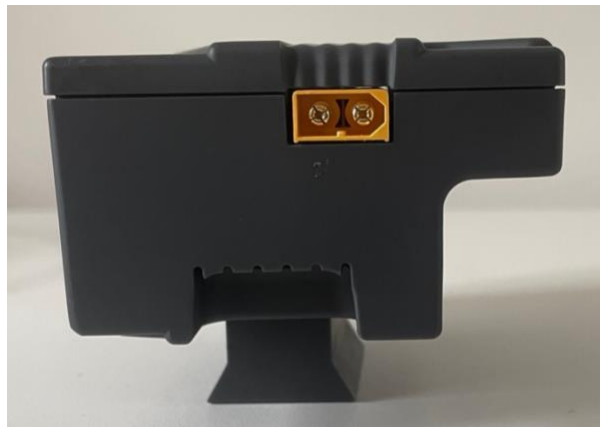
Figure 15. AStarBox with finder foot attached to the aluminium puck on the base of the box.
