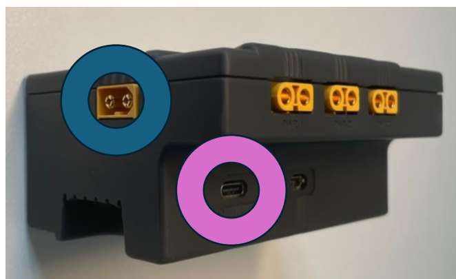
Figure 2. Location of input power. Provide 12 input via the male XT60 connector circled in blue, or 5v through the USB-C port circled in purple.
