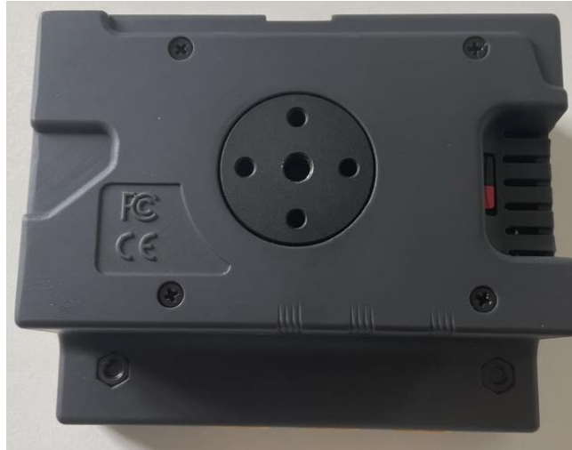
Figure 5. Base plate of the AStarBox. The centre hole has a ¼” thread whilst the four outer holes have M4 threads.
