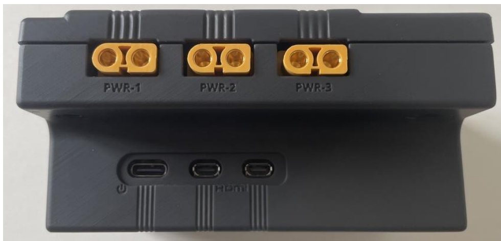
Figure 3. Three female XT60 connectors that can supply 12v at up to 5A to your devices. In the recess, there is the Pi USB-C socket and twin micro hdmi sockets.
