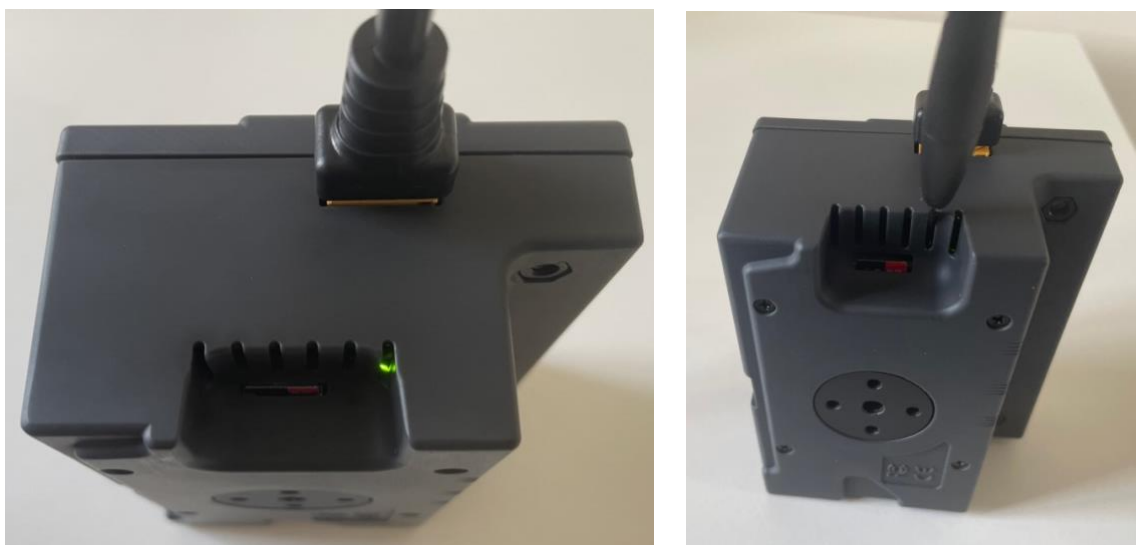
Figure 2. The LED status light is visible through the rightmost ventilation hole. You can access the push on/off switch through the second on the right ventilation hole using a thin tool such as a small screwdriver.
