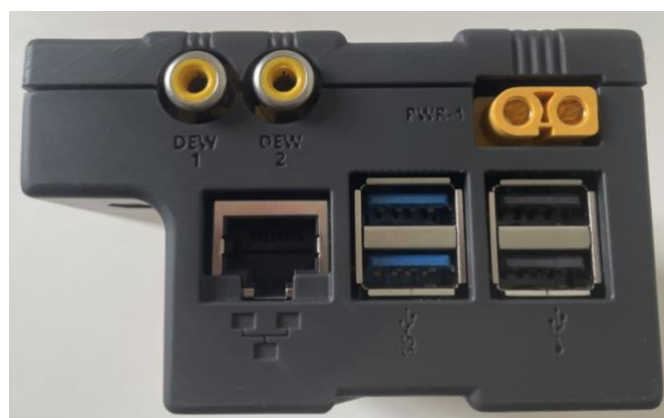
Figure 4. Final female XT60 power socket and the two dew heater outputs. Below these are the ethernet socket, twin USB 3 sockets (in blue) and twin USB 2 sockets (grey).
