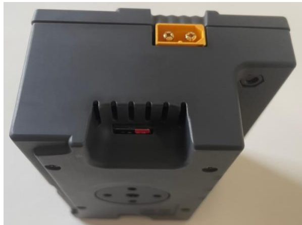
Figure 1. Location of 12v power input and microSD card slot below the ventilation holes.
